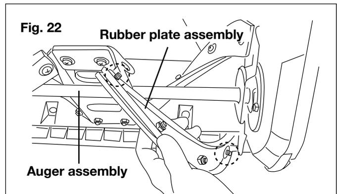
2. Loosen the middle two sets of nuts and bolts to detach the worn rubber plate from the metal frame (Fig. 23).
