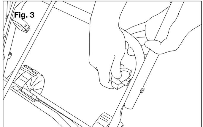
3. Secure the connection of the middle frame to the upper frame by fastening the second set of joint fixing T-bolts and knobs on each side (Fig. 4).
