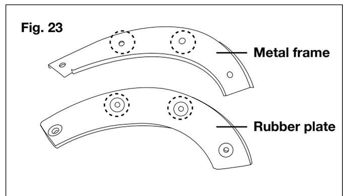
3. Attach the new rubber plate onto the metal frame by replacing and tightening the middle two sets of nuts and bolts (Fig. 23).
