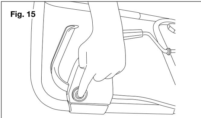
2. While depressing the safety switch button, pull the ON/OFF switch lever toward you. Once the machine powers on, release the safety switch button and begin operation (Fig. 16). The machine can only be started by depressing the safety switch button first, followed by squeezing the ON/OFF switch lever; reverse operation will not start the machine.
