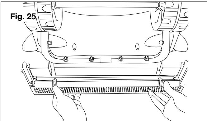
3. Install the new scraper bar and fasten it securely to the snow thrower with the two screws (Fig. 26).
