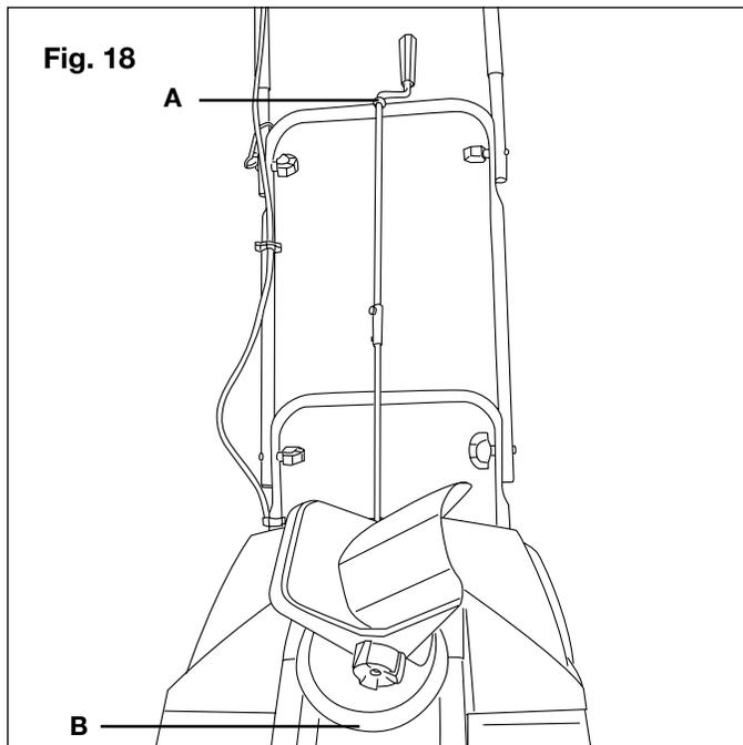
**NOTE:** A little lubricant, such as WD-40, will provide a smoother operation of the chute (spray at points A and B as indicated in Fig. 18).
